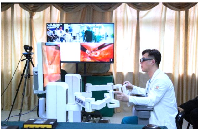
FIGURE 1 Master operation side of telesurgery. The chief surgeon controls the master operation terminal of the telesurgical robot and remotely performs surgical manipulation through the network transmission device.
